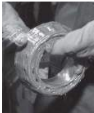
Fig. 23. Grease can easily be packed by hand.
